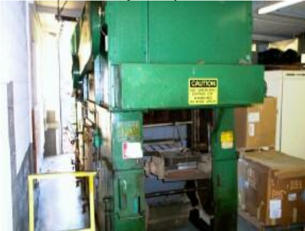
Old Crossrod Vapor Degreaser
