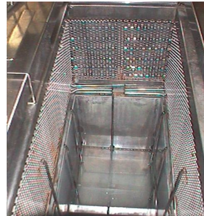
Freeboard & Primary Cooling Coils
